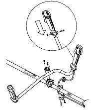
· The handlebar mounting must be fitted between the arrows on the shaft. Tighten the screws with a hex wrench.
