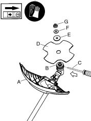
Hook the blade guard/combination guard (A) onto the fitting on the shaft and secure with the bolt.
