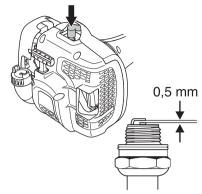
**CAUTION!** Always use the recommended spark plug type! Use of the wrong spark plug can damage the piston/cylinder. Check that the spark plug is fitted with a suppressor.
