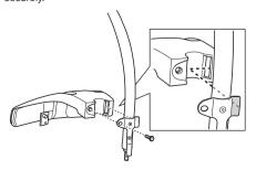
Fit the dust cup on the shaft. The nut must be completely covered by the dust cup.
